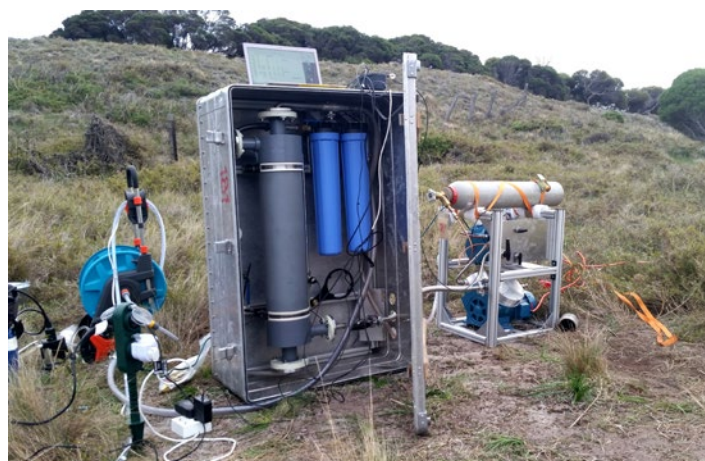
Field-going vacuum system used to collect samples.
